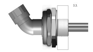
5. Tighten the Conduit Connector (4) onto the conduit to complete the installation.
